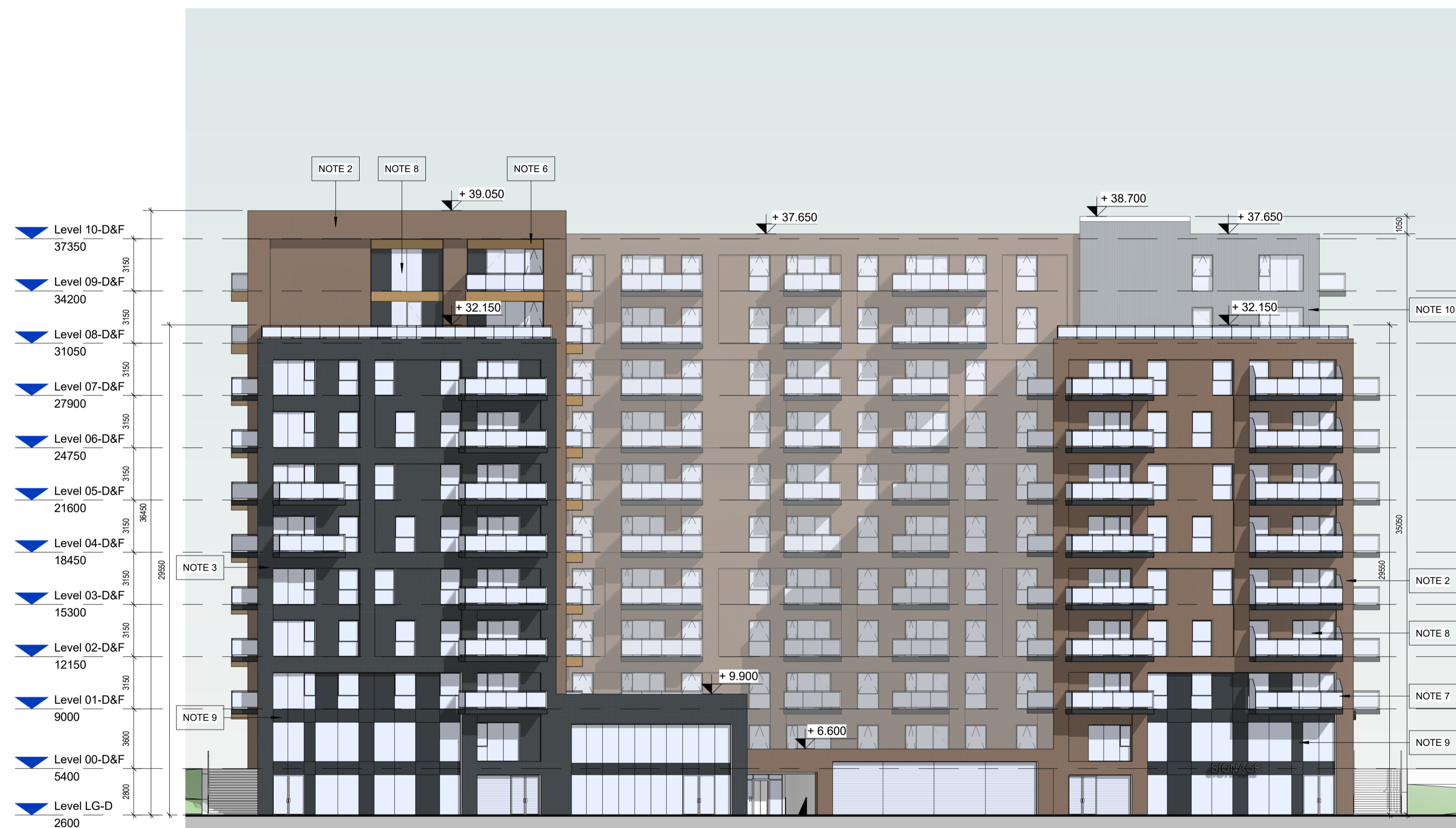
1 BLOCK D-SOUTH ELEVATION 1 : 200
